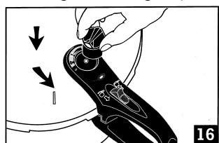
4. Lift the valve upwards and out. Clean as instructed above.
