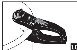
2. Gently lift the operating valve upward, not more than a quarter of an inch (Fig. 15).
