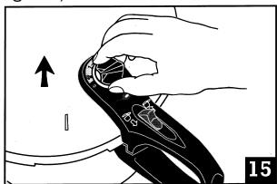
3. As you are pulling the valve up, keep trying to turn it to the left, counterclockwise, toward the picture of the circle with the line through it. You are looking for a groove, once you find this groove the valve will allow you to turn to the unlock position (picture of the circle with the line through it, see Fig. 16).
